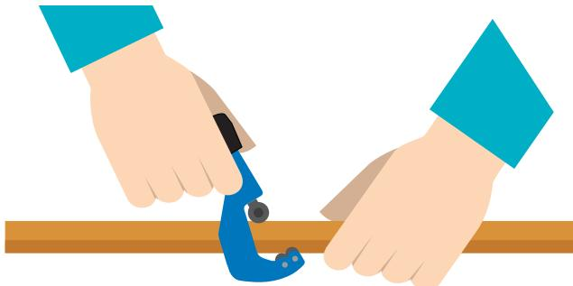
**en** Cut the copper tube using the **supplied** tube cutter. Do **NOT** use a hacksaw or reciprocating saw as this creates a rough surface that may damage the o-ring.
