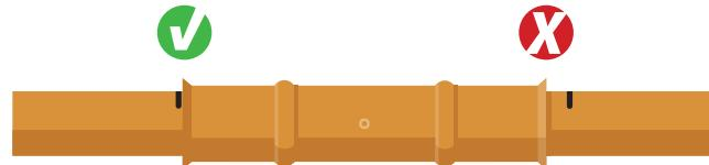
**en** Push the fitting onto the tube. Use the mark to assure insertion depth and secure fit.
