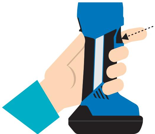
**en** Press and hold the trigger on Crimping Tool to calibrate.
