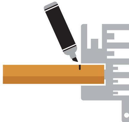
**en** Use the depth gauge provided or the chart at right to determine the proper insertion depth. Mark the tubing with a permanent marker to indicate proper insertion depth on every tube.
