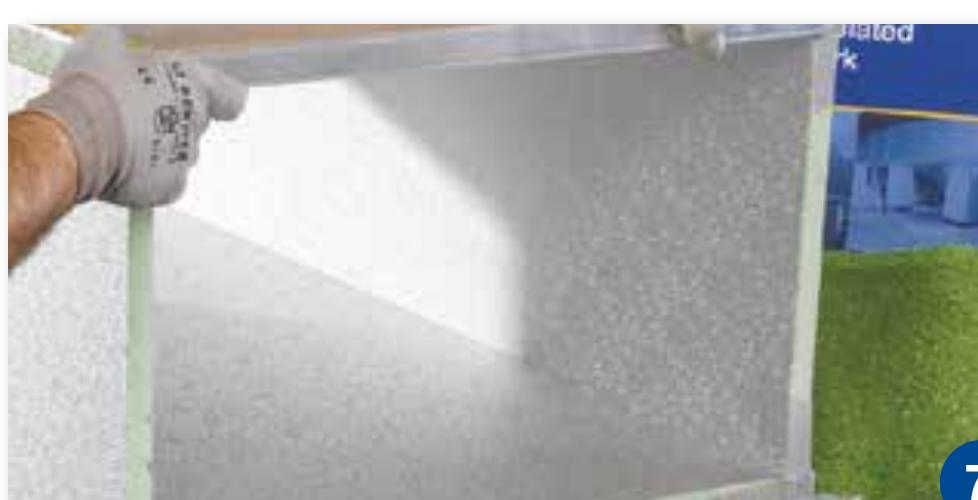
1. Using the nylon marking pencil, the shapes and dimensions of each duct can be easily traced
